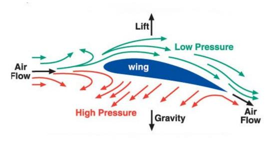
Figure 2: Forces in Flight
